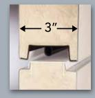
A Full Thermal Break is used in the tongue-and-groove construction of all 5800 series doors. This rigid vinyl extrusion seals the joints and eliminates metal-to-metal contact, which limits the transfer of temperature.
