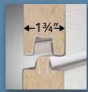
A Full Thermal Break is used in the tongue-and-groove construction of all 700 series doors. This rigid vinyl extrusion seals the joints and eliminates metal-to-metal contact, which limits the transfer of temperature.
