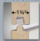
A Full Thermal Break is used in the tongue-and-groove construction of all 5700 series doors. This rigid vinyl extrusion seals the joints and eliminates metal-to-metal contact, which limits the transfer of temperature.
