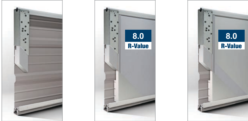
Pan - No Insulation Pan Polystyrene Insulation with high impact vinyl back cover Pan Polystyrene Insulation with 27gauge steel back cover
